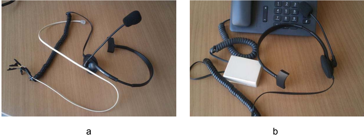
Figure 2. a) The first cheap headset that was “destroyed” while trying to make it compatible with the telephone device b) After finding the correct cable sequence, a more elegant method was used for the rest headsets (reorganizing of the internal cables was done inside the white boxes while keeping the cable jacks intact)
